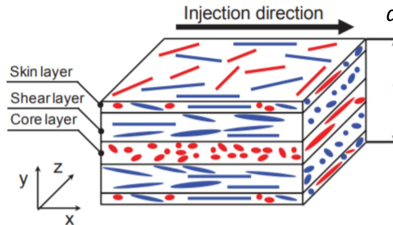
*Example of orientation tensor element along thickness  $t$*
