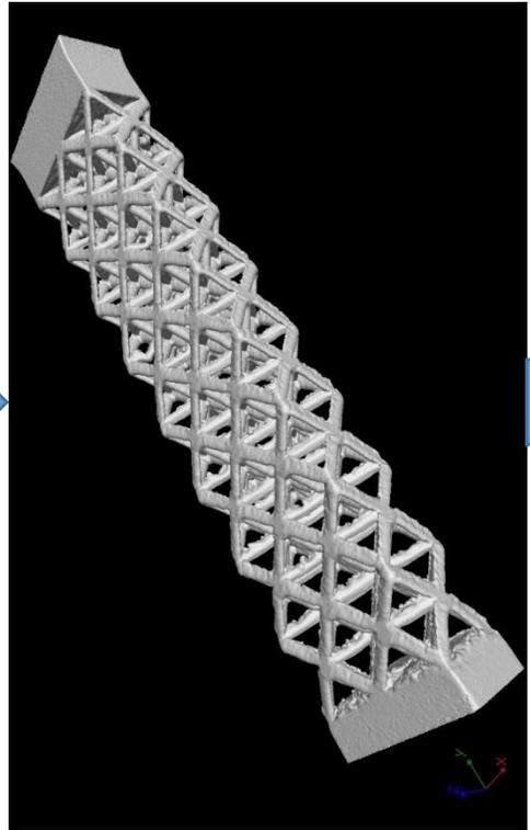
Mesh conversion with 15  $\mu\text{m}$  tolerance
