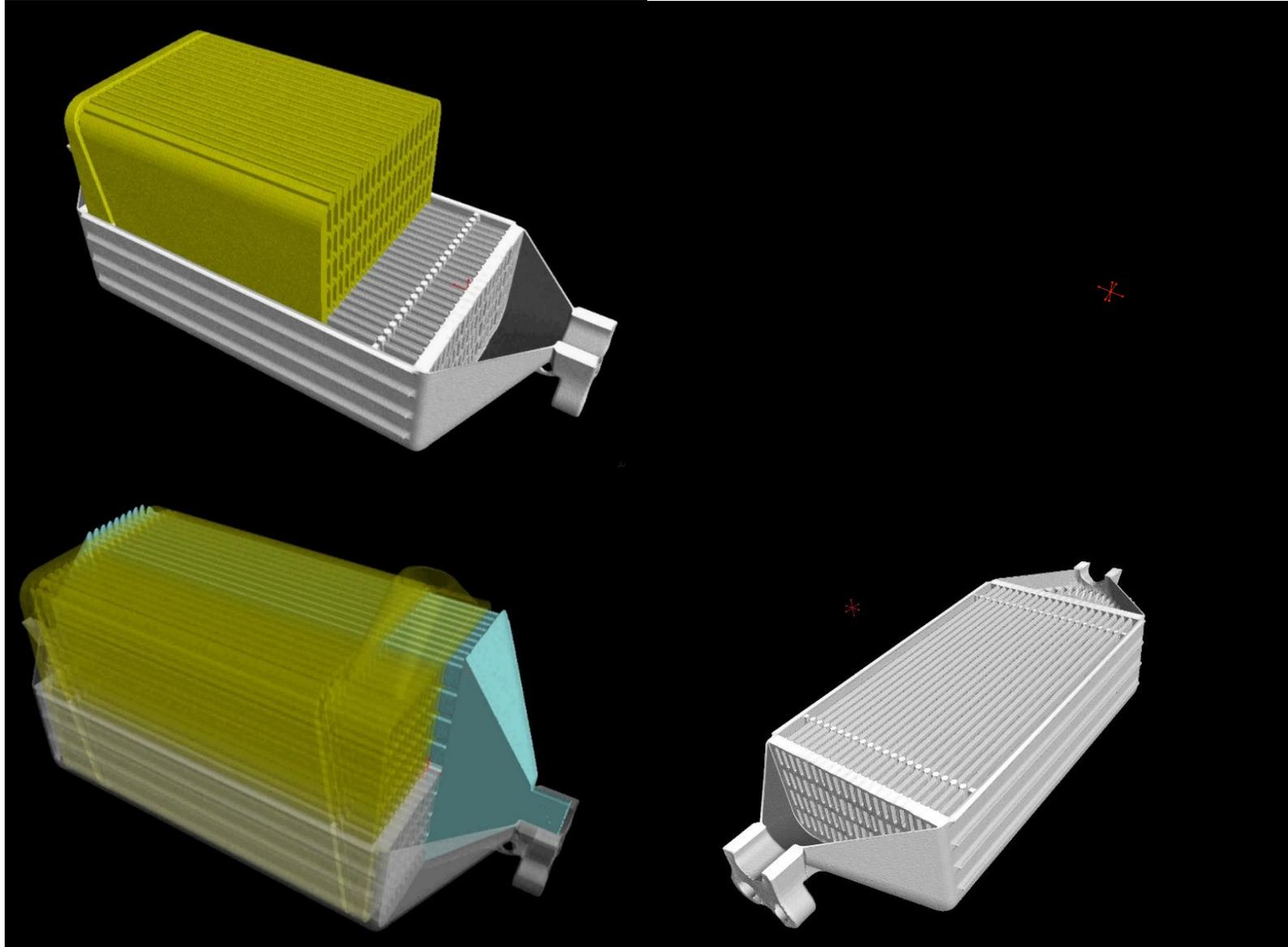
Exchange of 12 kW and compared to its conventional equivalent, it takes up 1/5 of the space. Walls of 0.4 mm thickness
