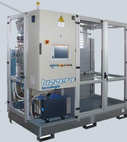
Computerized Burst test up to 100 MPa
