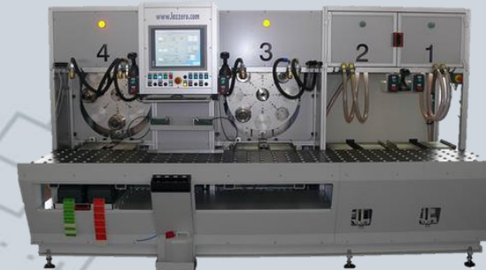
Computerized Burst test up to 100 MPa
