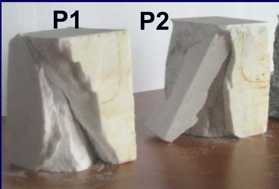
Specimens P1 and P2 in Carrara marble following compression failure.
