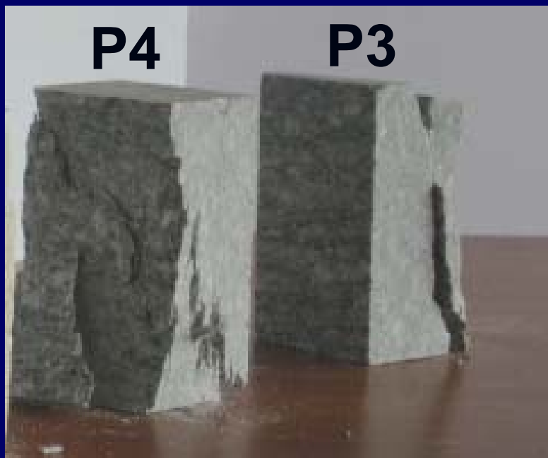
Specimens P3 and P4 in Luserna granite following compression failure.
