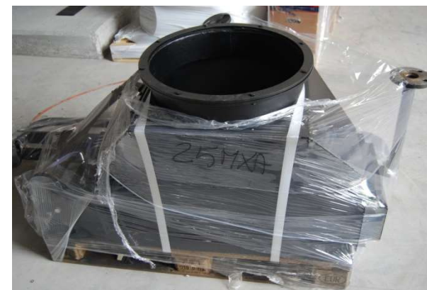
Economizer on flue gases (+ 3-4% efficiency increase)
