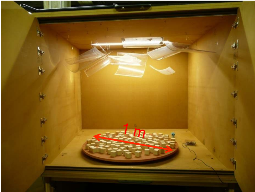
Sound scattering measurements
