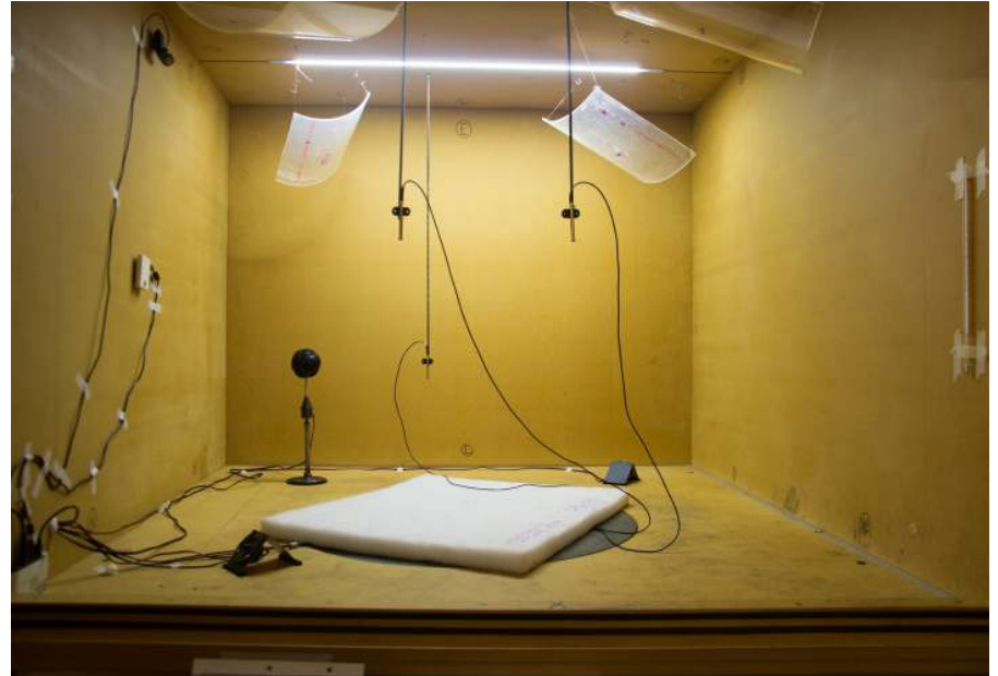
Sound absorption measurements
