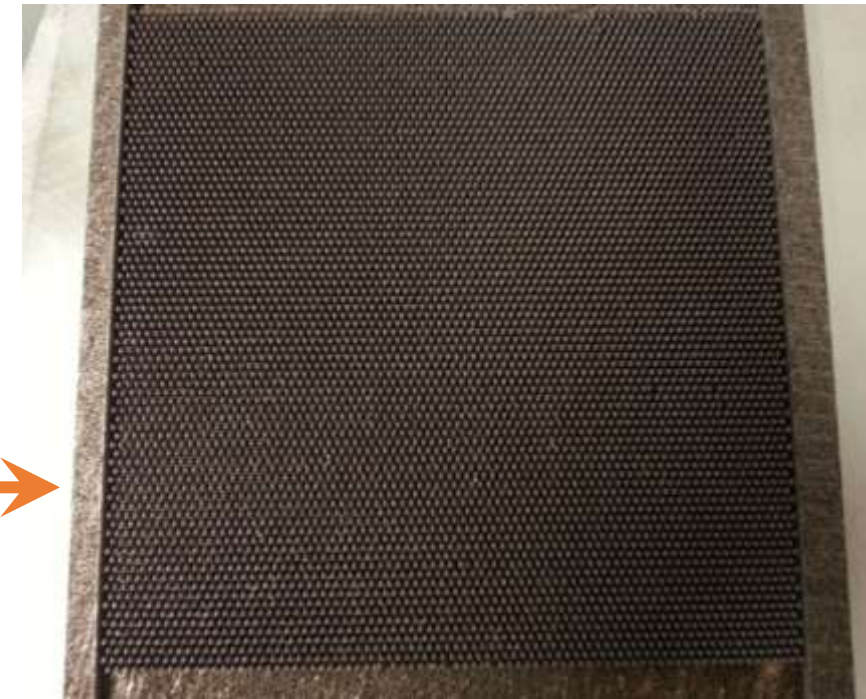
For each layer 6320 elliptical fins
